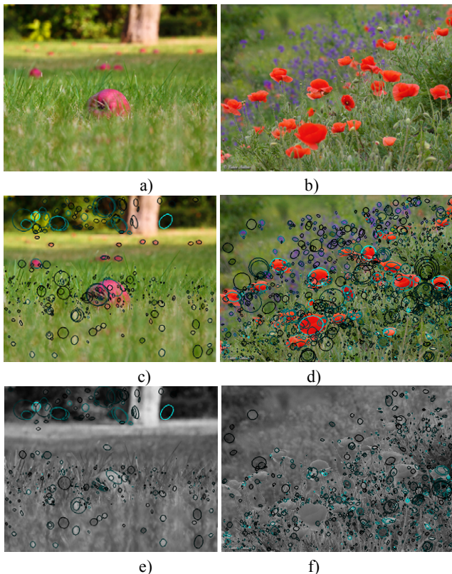
Figure 4: Comparison of results obtained from the proposed algorithm ((c) and (d)) and detection after conversion to grayscale ((e) and (f)). Response threshold is 0.75. After conversion to grayscale most noticeable color features are missed.
